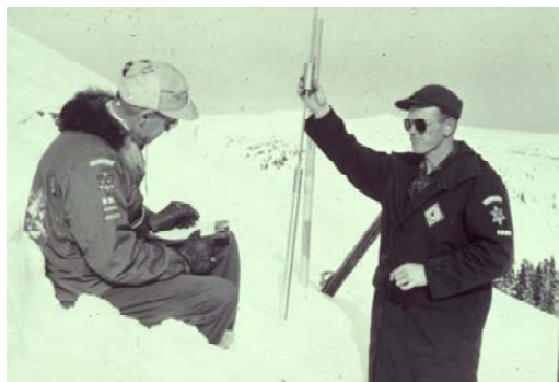
Operating a ram penetrometer at Alta
